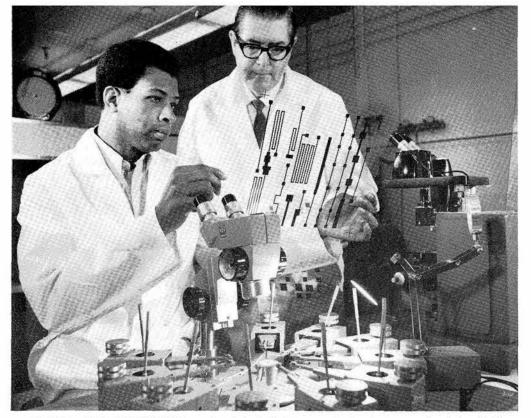
RESISTOR AND CONDUCTOR mask of hybrid integrated circuit is examined by (left) Ike Davis and Bob Noble (both 8182) in SLL's new microelectronic lab. The lab will help to keep engineers up-to-date on advances in microminiature hybrid integrated circuits.
